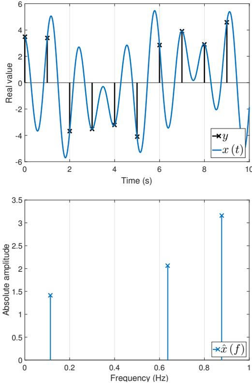
Figure 1. Time and spectral representation of a signal  $x$  following the spikes model with three spectral spikes and its measurement vector  $y$  when taking  $n = 10$  observations at a frequency  $f_S = 1\text{Hz}$ .
