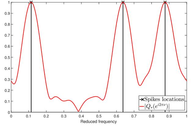
Figure 2. The optimal dual polynomial  $Q_*$  obtained by solving Program (5) when retaining entries of  $y$  with indexes in the set  $\mathcal{I} = \{0, 3, 4, 6, 8, 9\}$  of cardinality  $m = 6$ .  $Q_*(e^{i2\pi\nu})$  locates the frequencies of the signal  $x$  by reaching modulus 1 whenever  $\nu \in \frac{1}{f_S}\Xi$ .
